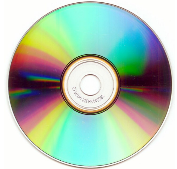
The grooves of a CD can be used as a diffraction grating
