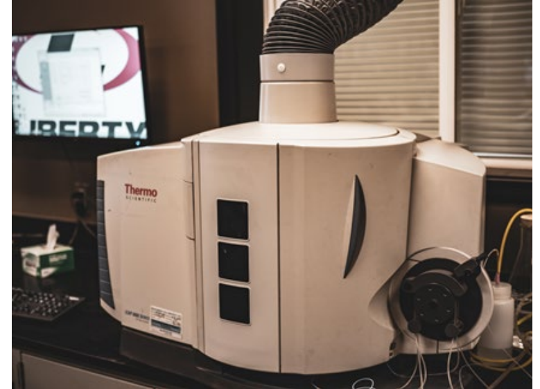
Image of our ICP-OES in Williston. We have a total of 3 units across the country
